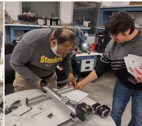
Marc and Pablo aligning y-linear belt drive guide with x-linear guide
